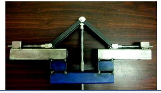
Prototype of a base isolator of vertical seismic vibration (Mochida et al., 2014)
