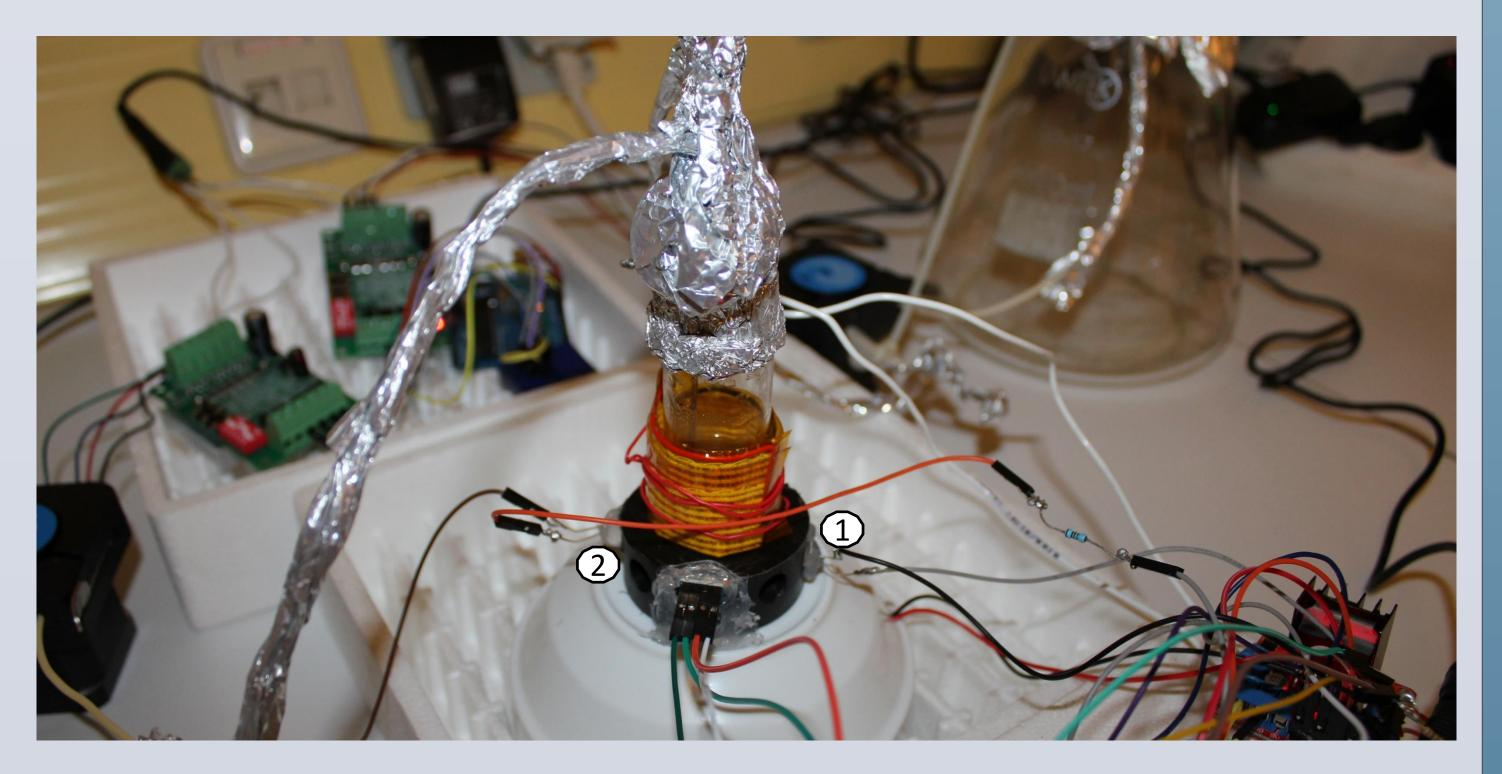
The whole system is maintained by two Arduinos, one is for controlling peristaltic pumps to allow 6 ml liquid circulation in 60 minutes.
