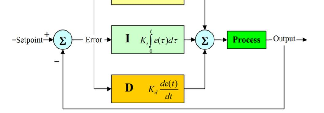
We used mainly two control systems in the project. First one is controlling the angular velocity values of the wheels and e used just proportional control. Furthermore, we used PID control for gyro sensor's values for which we used the integral and proportional controls. We prevent the slippage, which occurs due to lack of friction constant, of the robot by calculating and controlling the Gyro values.
