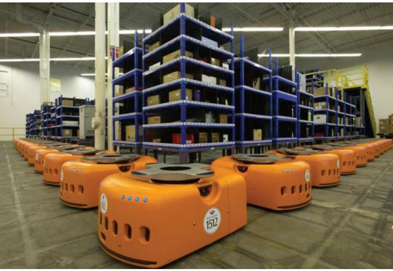
Kiva system used in warehouses which use autonomous robots to enhance the shipping time, quality and cost by commanding them to bring the storage pod to the packing personnel
