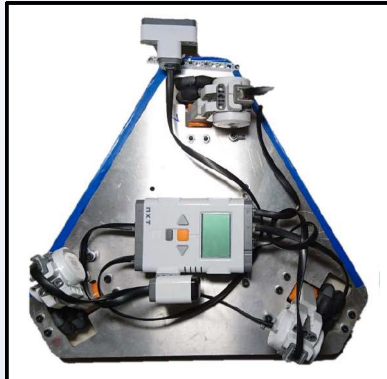
Figure 2: The omnidirectional LEGO robot's bird's-eye-view photograph.
