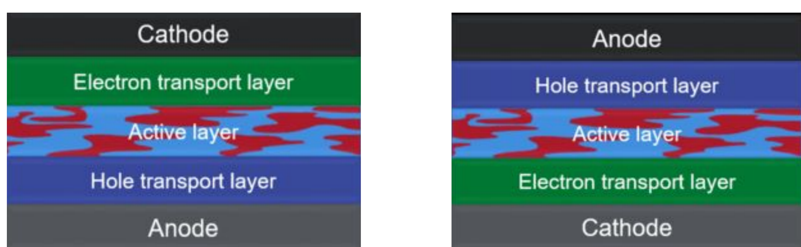
Fig. 3. Conventional (left) and inverted (right) structure of solar cells (Ossila, n.d.)
