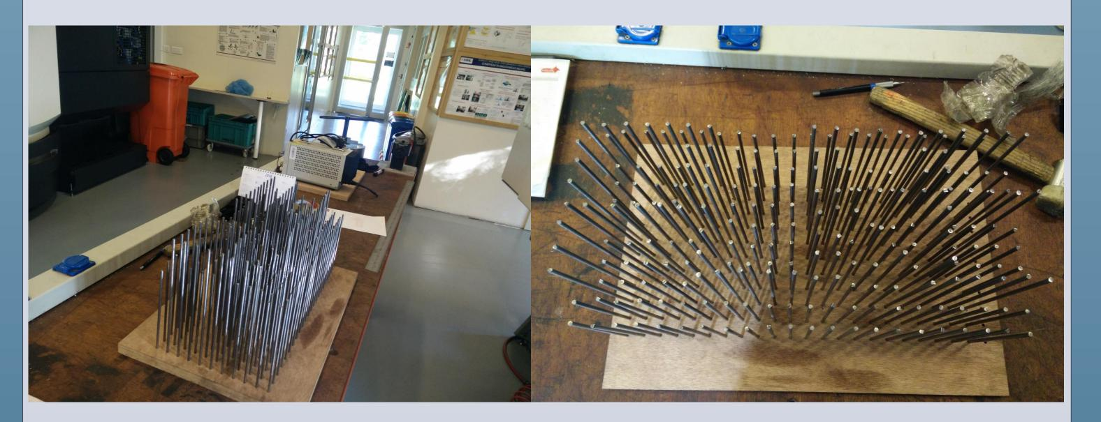
• We drilled holes in the wooden surface in the machine shop and then inserted the rods in the holes after which we attached our wooden surface to the electric motor.
