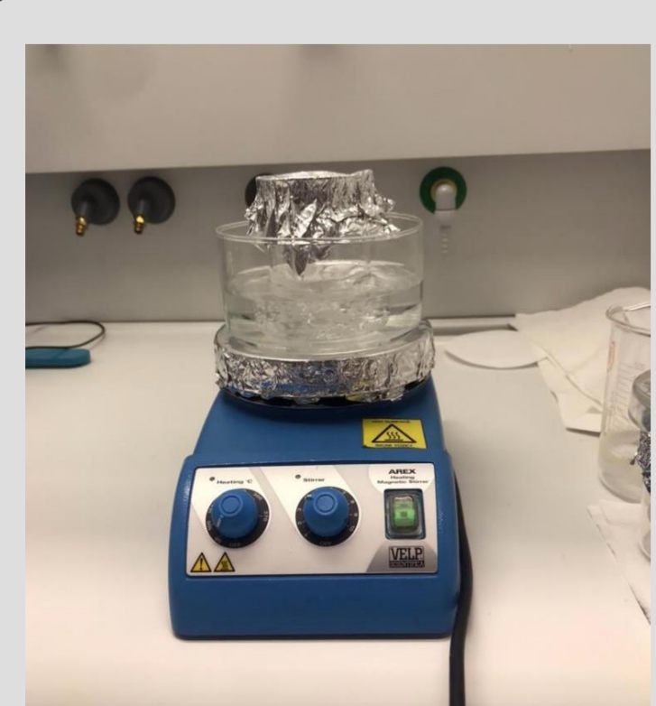
Figure 1: The beaker with PCL left to mix at 40°C for 24 hours
