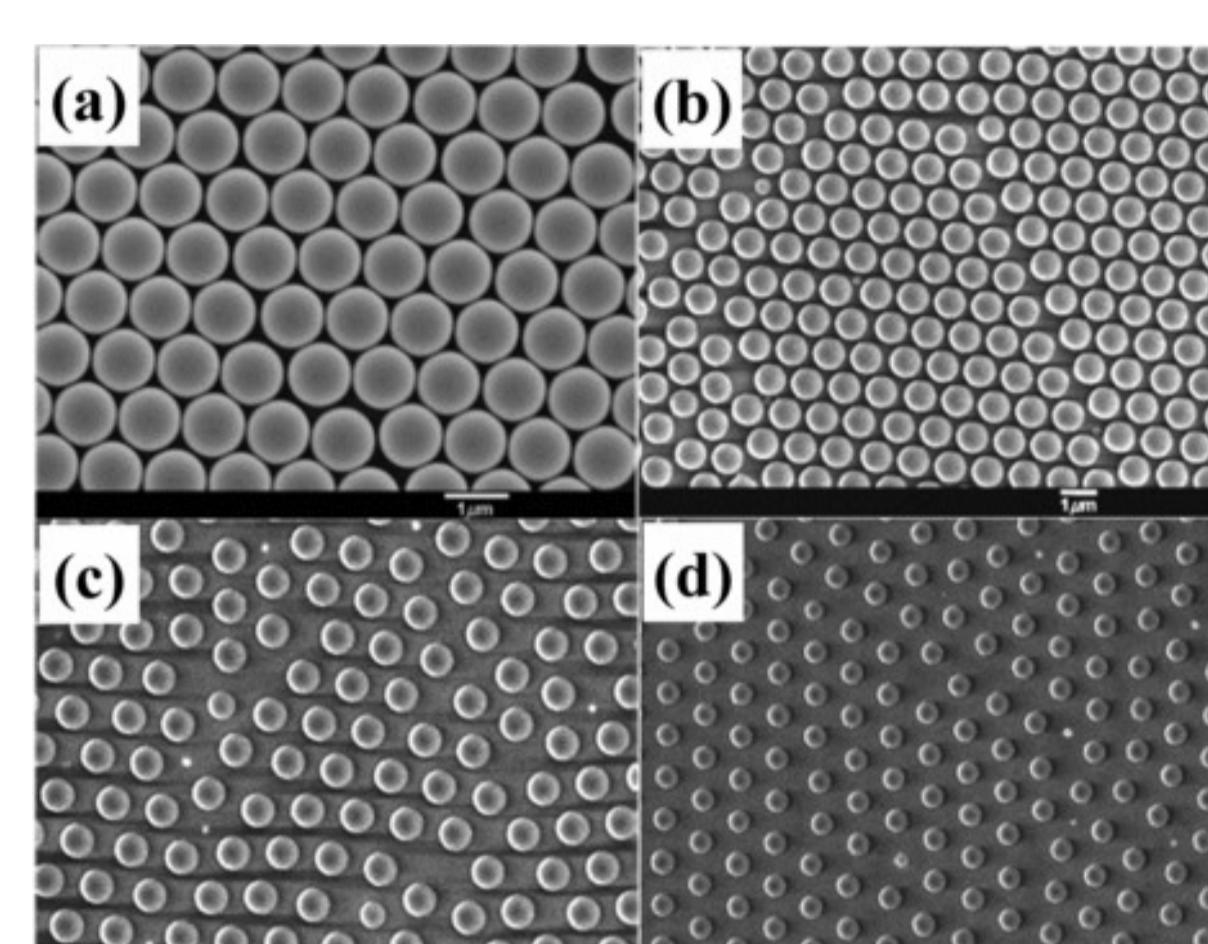
“SEM images of 2D PS colloidal crystals. (a) Initial 1000 nm microspheres in closely packed arrays, (b-d) non-close-packed colloidal crystals by plasma etching 4, 6, 7 min, respectively.”
