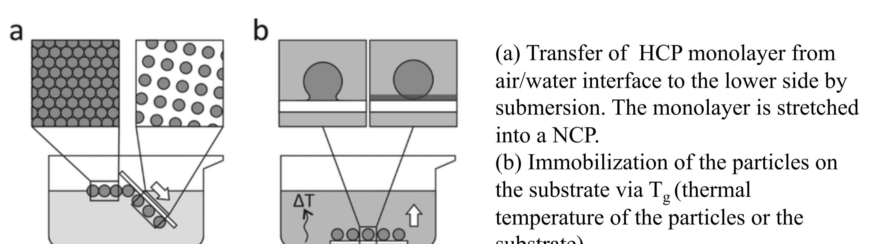
Experimental setups of stretching method:
