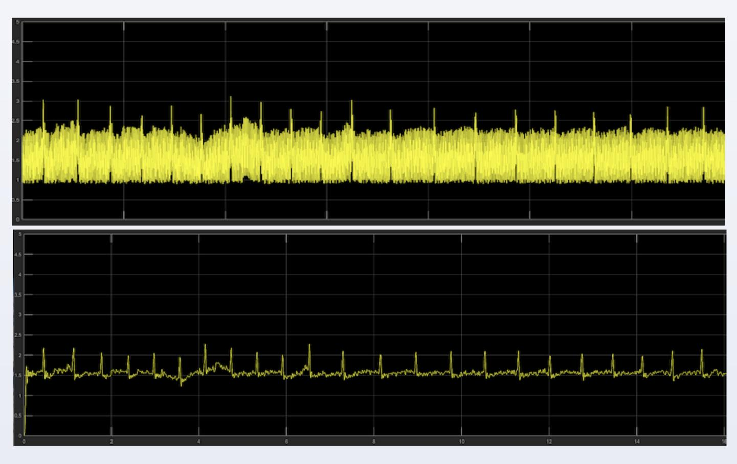
Arduino Uno is used for A/D converter and MATLAB is used for processing the data in PC. The raw data from the circuit at the top image is very noisy. To clear the noise, a digital Notch filter at 50 Hz is applied. The second image is the filtered signal and QRS complex of the heart is clearly visible. Also P-T waves are distinguished in a close look but they're noisy. Graphene-coated textile electrodes are shown in the figure below and similar results are obtained using them.
