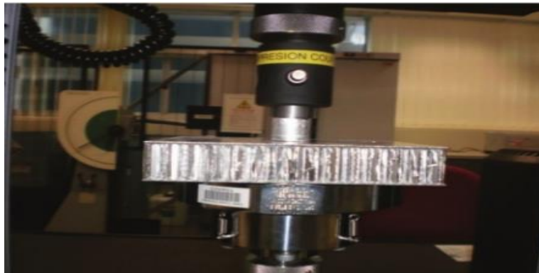
Fig.12. Perimeter Shear Testing
