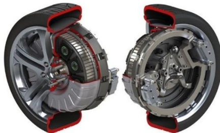
Figure 1: In Wheel Motor (Retrieved from https://motorwallpapers.org/protean-hub-motor/ )
