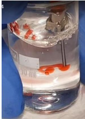
**Figure 7.** Testing the suitability of 18% Pluronic F127 supporting bath for bioprinting of alginate.
