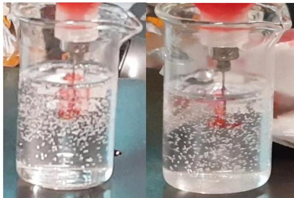
**Figure 9.** Testing the suitability of 21% and 22% Pluronic F127 supporting bath for bioprinting of alginate.
