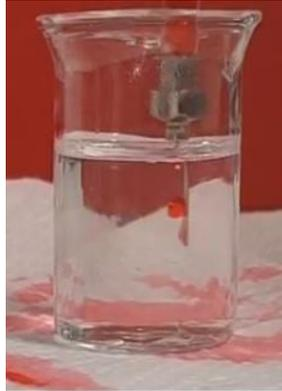
**Figure 6.** Testing the suitability of 16% Pluronic F127 supporting bath for bioprinting of alginate.
