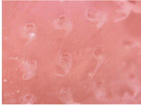
Figure 5: Microscope View of Failed PLC Microneedles
