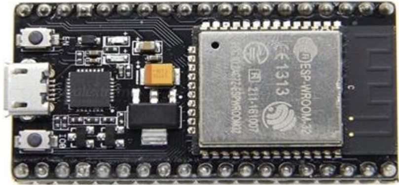
Figure 2. NodeMCU ESP-32S development board.
